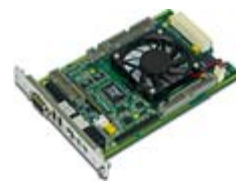
MIC580 3U 4HP Mezzanine Interface Card
