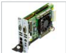
MIC580 with cooling fan.
